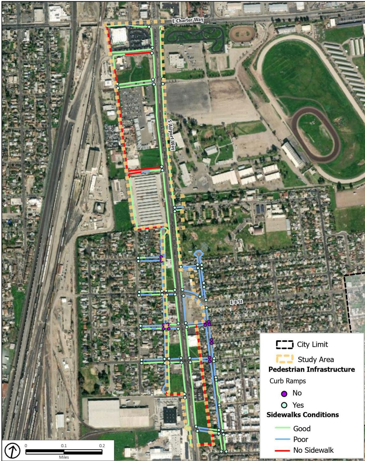
Figure 5: Sidewalk Conditions in South Airport Way
