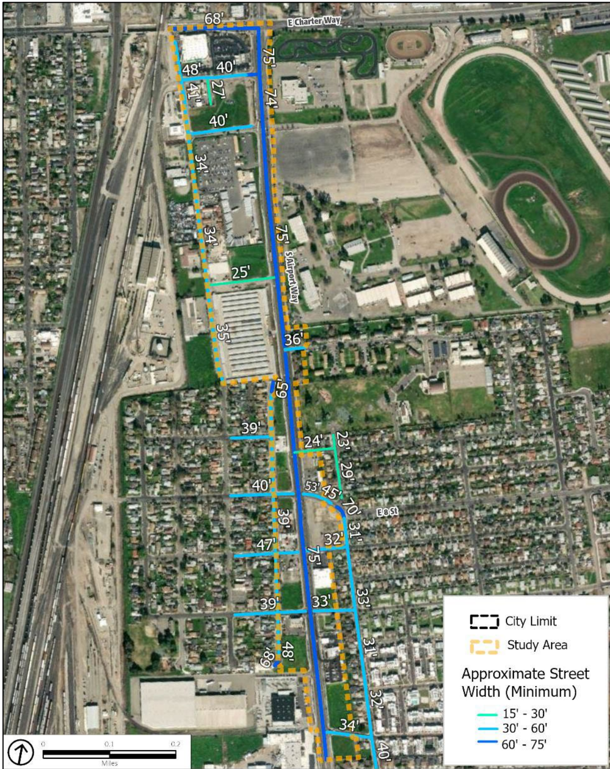
Figure 6: Minimum Street Widths in South Airport Way
